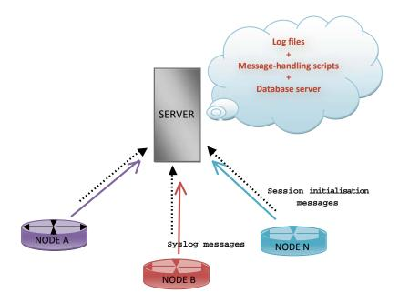
Figure 1. Schematic of network monitoring setup on UI network.
